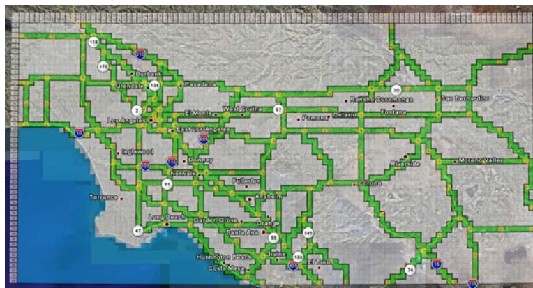
FIGURE 1 Los Angeles, California metropolitan area showing modeling grid structure (not including “buffer zone”) and major expressways as laid out in the grid format
